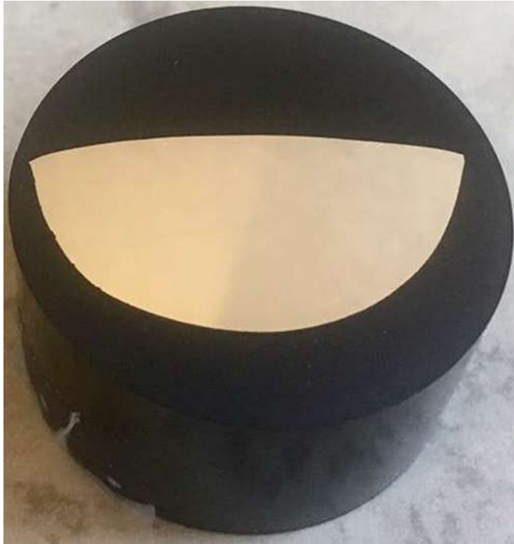
Figure 9 – 1795 O-105 End Piece Mounted In Bakelite
